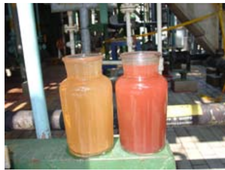
Sample test from primary scrubber vessel
